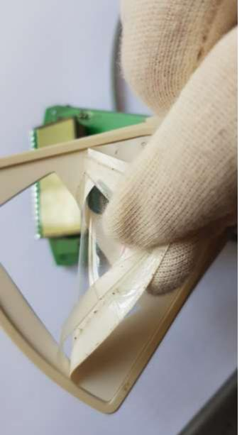
Remove the Keypad no problem if destroyed while removing
