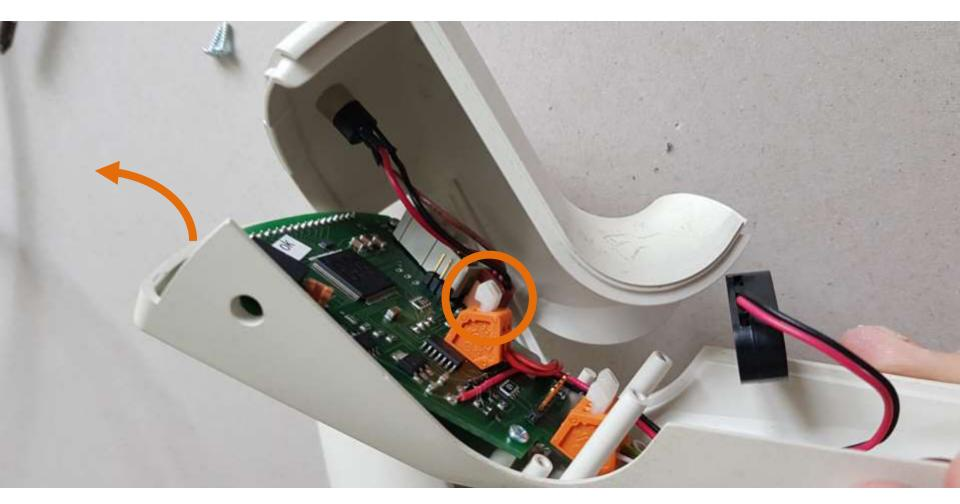
Bend the casing a bit to open it
