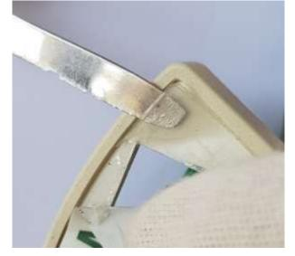
Be sure to remove both level of the keypad
