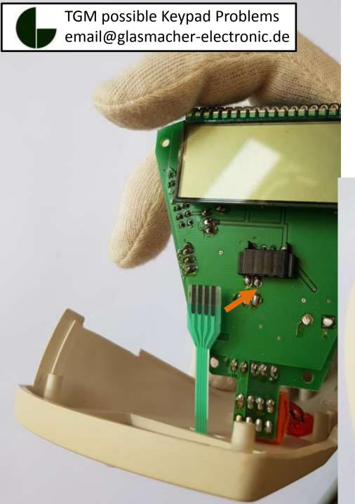
Reconnect the foil cable with the plug on the circuit board with a tweezer
