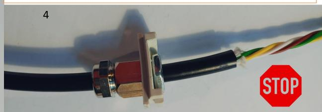
Pull the cable through the metall clamp till about 1cm is out of the unisolated cable – reconnect the metall clamp – a bit of water on the cable makes it easier
