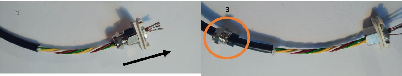
Put the 4 loose ends without the cable tie through the metall cable entry
