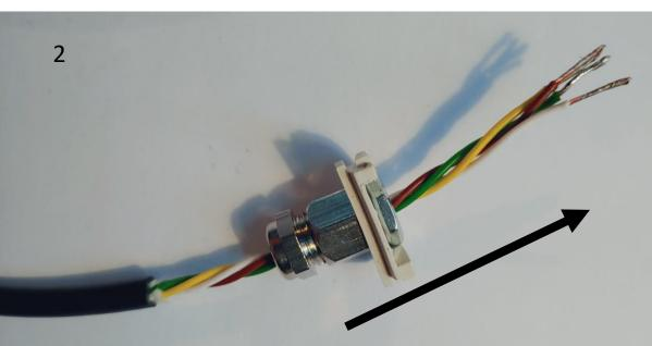
Open the metall cable entry and put the outter part with the rubber a bit over the isolated black part of the cable
