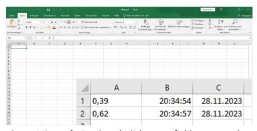
Open Microsoft Excel and click on a field to start the listing of the measuring results. The Export to Microsoft Excel is now set and starts in the field clicked (here A1). The results of every measurement will now be shown in the open Excel sheet. The first column will be the TGM result then the Time (hh:mm:ss) and then the date.
