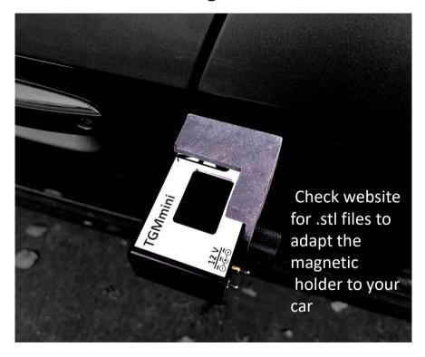
Use the magnetic holder to mount the TGMmini near the car door on flat surface car bodies.
