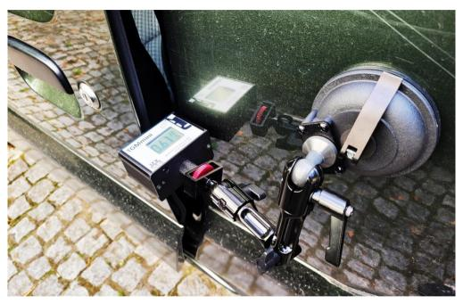
Use the 1/4"-20 UNC tripod thread (#4 on picture at page 2) to mount the TGMmini to any available camera mounting systems or tripods. For example the <a href="Skier Prosystem">Skier Prosystem</a> 3d Vari Arm.
