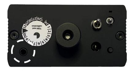
One way to export the results to your PC is via serial jackcable. You find the serial cable jack at the bottom side of the TGMmini.
