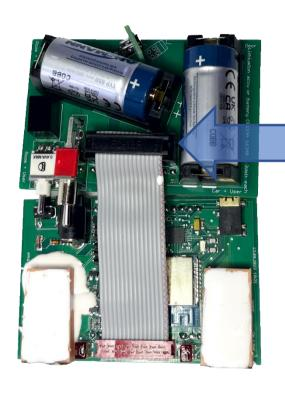
Before removing the batteries you can disconnect the PCBs by pulling the plug on the battery PCB.
