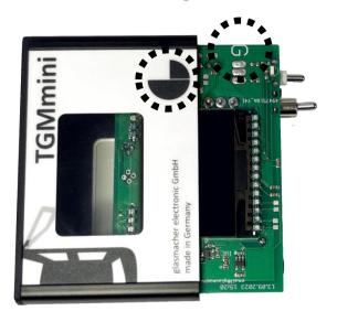
The TGMmini has two PCBs connected with a cable. Remove the PCBs gently from the casing.
