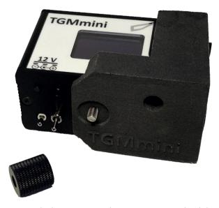
To mount and dismount the magnetic holder, unscrew the 1/4"- UNC Adapter and pull the device off the holder. You can than use the 1/4"- UNC Adapter or the M5 thread to mount the TGMmini.
