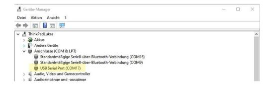
To export the Data to a terminal program for serial communication (Hterm; Microsoft Data Streamer etc.) first identify the TGMmini COM-Port in the device manager (here COM17).
