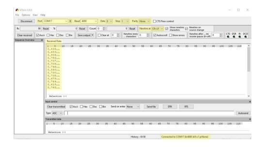
Open the terminal program and indicate the COM-Port (Page 31). To receive the UART Data, the Baud Rate has to be set at 4800, Data 8, Stop 1, Parity None. Set newline at carriage return and line feed (CR+LF). The Data comes in ASCII. The data export from the TGMmini to your terminal program is now set.
