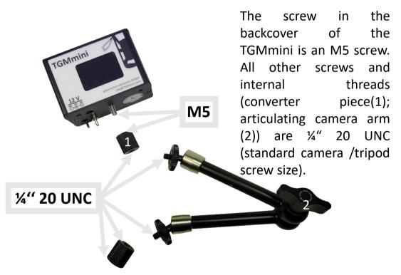
Therefore nearly all common tripods and camera arms available on the market can be used to mount the TGMmini on a vehicle or other objects.
