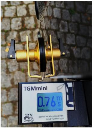
If the measured car door is not ferro magnetic, you need a measuring edge.
