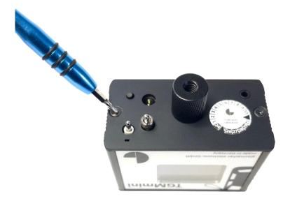
To change the batterys you can open the TGMmini on the side where the push button, the switches and the power plug are located. Use a Torx 10 screwdriver to open the casing. Do not open the other side. The aluminum screws are very delicate.
