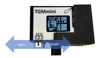
In Measuring Mode: Use Switch (5) to insert the result of the closure:
