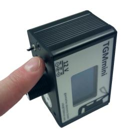
Turn the TGMmini ON by pressing the pushbutton (#2 on picture at page 2) recessed in the back of the housing.
