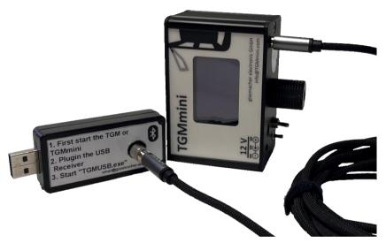
Connect the Serial jack-cable to the TGMmini and to the USB Adapter to connect the TGMmini with your PC.
