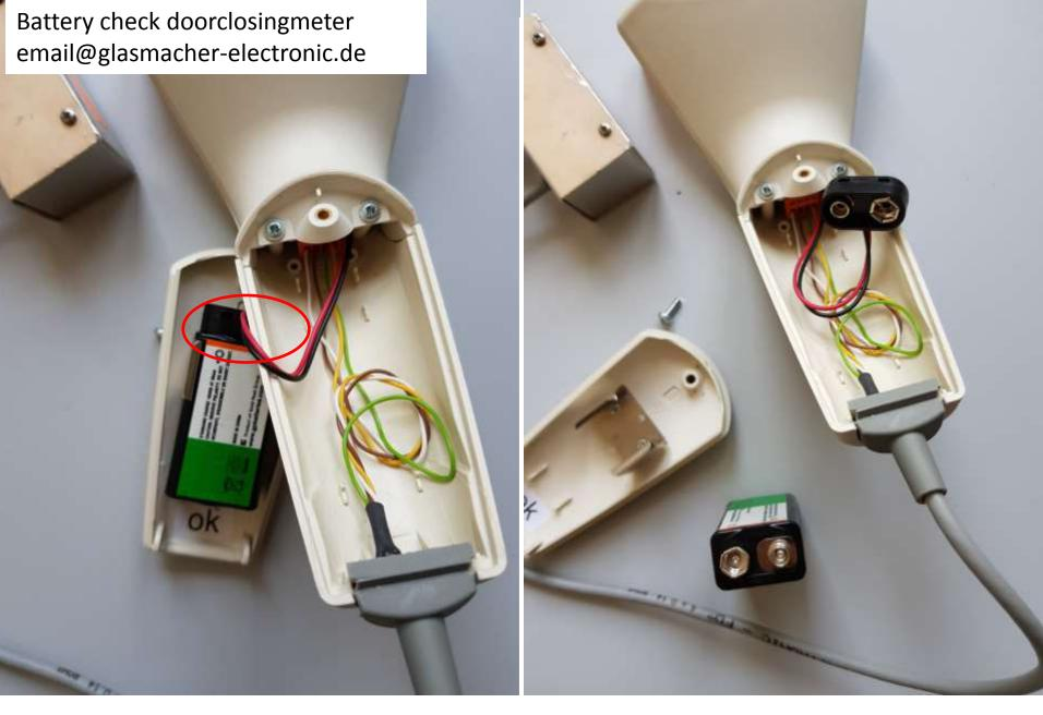
Check if battery/accu is connected properly to the battery clip
