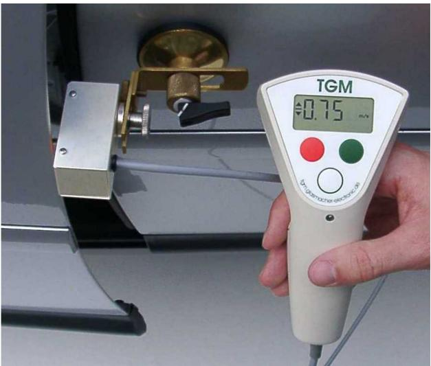
It is advisable to mount the sensor on a stand which is adapted to a particular car model with a stop bar so that it can be installed quickly with precise distance from the door edge to the body for serial tests and measurements. The sensor is fixed and aligned to the body so that the door edge passes the sensor at a distance of less than 10 mm. The red arrow points in the direction of the car body, i.e. in measuring direction.
