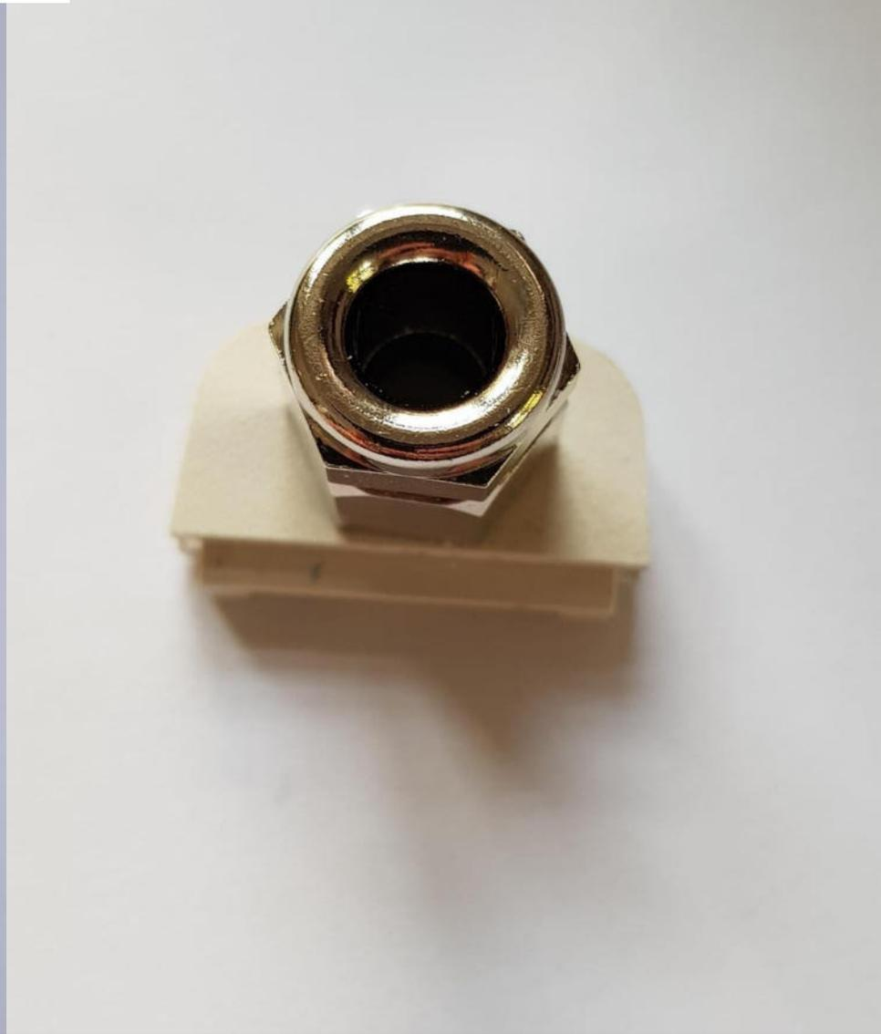
Because of repeated problems with the cable grommet we changed it in early 2018 from glueing to clamping – please contact [email@glasmacher-electronic.de](mailto:email@glasmacher-electronic.de) so we can change for you in Germany or send you the metall clamp free of charge so you can change
