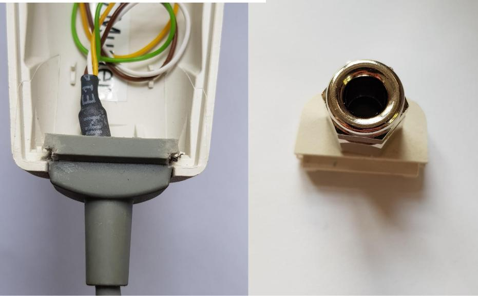
Because of repeated problems with the cable grommmet we changed it in early 2018 from glueing to clamping – please contact <u>email@glasmacher-electronic.de</u> so we can change for you in Germany or send you the metall clamp free of charge so you can change
